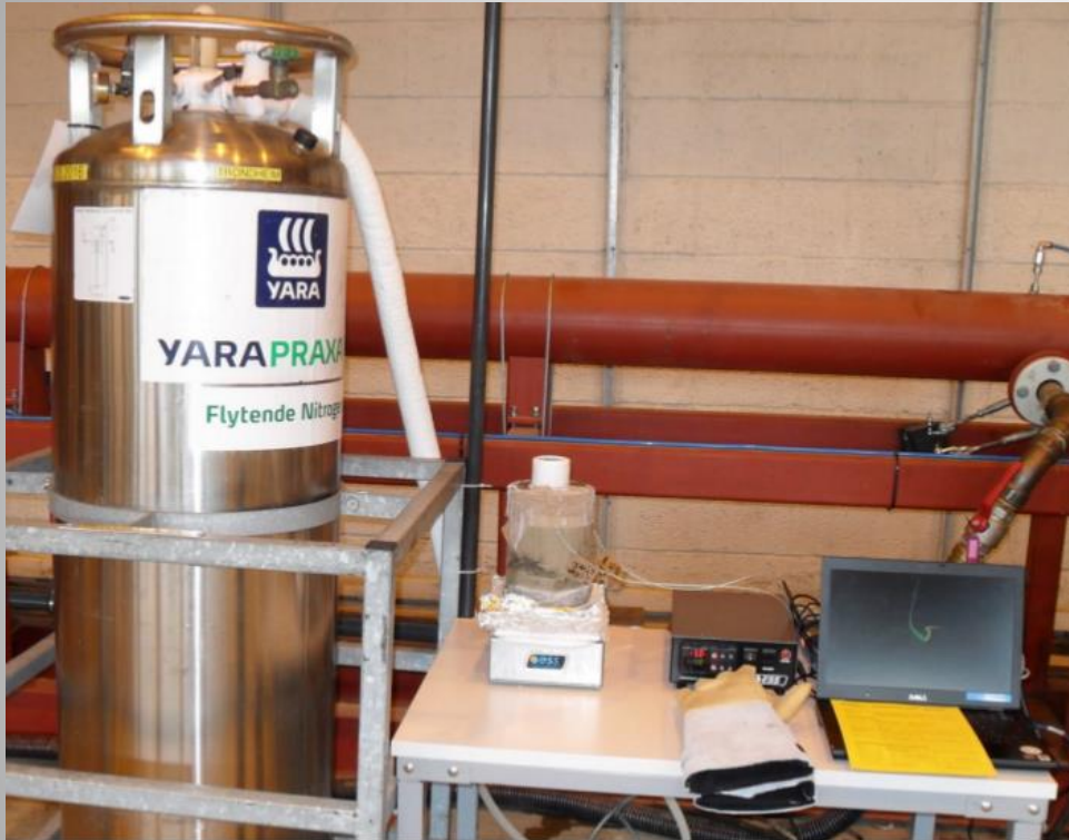
SINTEF Thermal cycling setup with liquid nitrogen tank and heating/cooling stage
